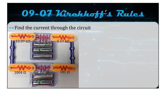
Loop Rule (starting top left going CCW)  $I(10090 \ \Omega) + 4.5 \ V + I(5170 \ \Omega) + I(101 \ \Omega) + I(1004 \ \Omega) = 3 \ V$   $16365 \ \Omega \ I + 4.5 \ V = 3 \ V$   $16365 \ \Omega \ I = -1.5 \ V$  $I = -9.17 \times 10^{-5} \ A = 91.7 \ \mu A$
